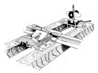
Model HB Sliding Derail is a heavy-duty derail designed for durability and to minimize stress on wheels and derail. It is operated from the side of the track with a stand that slides the shoe from the base to the upper (active) position. Pictured at left is model HB with a standard two-tie operating stand. Other types of stands are available. The stands require a connecting rod, and must be ordered separately. Weight (w/o stand) - 277 lbs.
