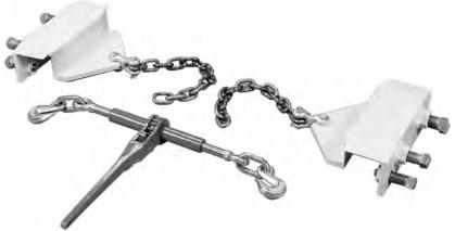
Rail-Pull brings rail back into gage after derailment so rerailing can proceed. Cars can freely pass over rail-pull clamp plates. Weight 76 lbs.
