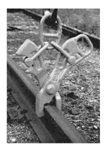
Clamping Rail Tong for crane rail 135 lb., 171 lb. and 175 lb. Load capacity 4000 lbs. Lift only—no dragging. Weight 60 lbs.
