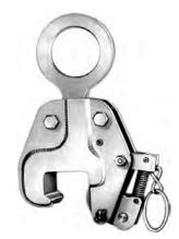
**Rail Tugger** has a self-locking wedge to tightly grab rail for easy pulling and positioning of rail lengths. Handles rails from 100 to 141 lbs/yd. Weight 40 lbs.
