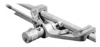
Hydraulic Rail Benders for light rails are the double hook type with a 25 ton hydraulic ram-pump or 50 ton ram with remote pump. They provide direct 90 degree pressure against the rail head between the hooks. The underlipped hooks of the frame have convex bearing surfaces to prevent crawling off the rail
