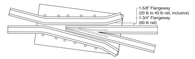
Welded Plate Frog Design 97 is recommended for use in mines, construction work and industrial plants where light rails are used.
