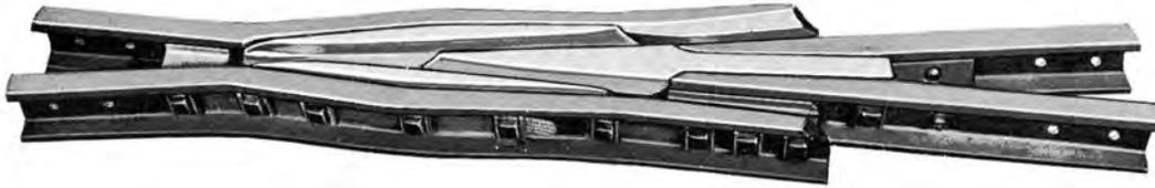
A **Railbound Manganese Steel Frog** is constructed with a manganese-steel body casting. This casting is fitted into and between four rails that are specially fabricated from standard tee rails. The assembly is fastened with heat-treated bolts. This type of frog is used for heavy and/or high-speed main line service, where the traffic is approximately equal on both sides of the frog.
