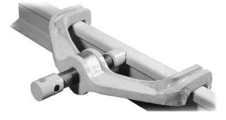
**Screw Type Rail Benders** for light rails are designed with double-hook style cast steel frame and provide direct 90 degree bearing to the rail head. The operator uses a steel bar to turn the screw.
