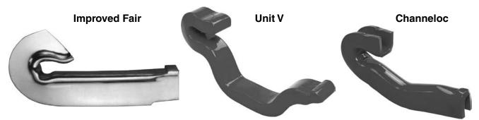
Rail anchors are manufactured in one-piece construction from spring steel or equal, heat-treated and designed to eliminate creepage of track. They provide a large bearing surface against both rail base and tie, avoiding undo cutting and wear, thus prolonging the life of wood ties. All anchors shown above are "drive-on" type anchors which are driven on using a standard spike maul.
