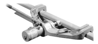
**Hydraulic Rail Benders** for light rails are the double hook type with a 25 ton hydraulic ram-pump or 50 ton ram with remote pump. They provide direct 90 degree pressure against the rail head between the hooks. The underlipped hooks of the frame have convex bearing surfaces to prevent crawling off the rail. The hydraulic benders are much easier to use than the manual screw type.
