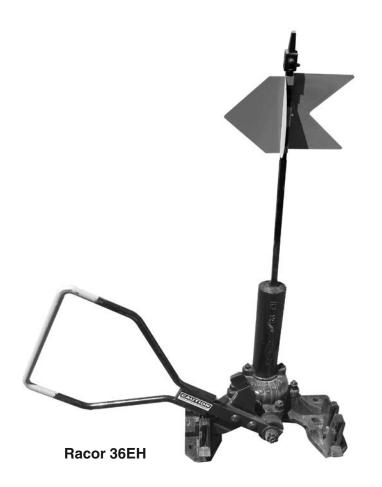
The **Racor 36E** and **36EH** are extraheavy-duty non-trailable switch stands for unrestricted use. Both models have identical base housing and operating parts. The 36E is most often used for yard operations, while the 36EH, with high mast and target, is suitable for mainline use.
